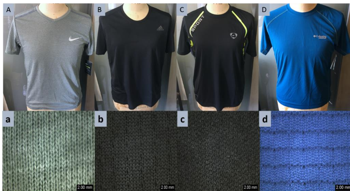
Figure 1. Appearance and fabric structure of fabric samples of different brands: Nike (A, a), Adidas (B, b), Laishilong (C, c) and Columbia (D, d).
